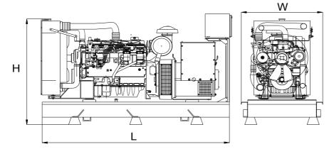
Length, L 2,4 m Heigth, H 1,7 m Width, W 1,15 m Weight, Total 1400 kg
