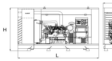
Length, L 3,25 m Heigth, H 2 m Width, W 1,2 m Weight, Total 1900 kg
