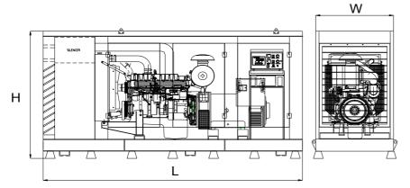
Length, L 3,25 m Heigth, H 2 m Width, W 1,2 m Weight, Total 2750 kg
