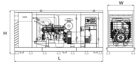
Length, L 3,25 m Heigth, H 2 m Width, W 1,2 m Weight, Total 2750 kg
