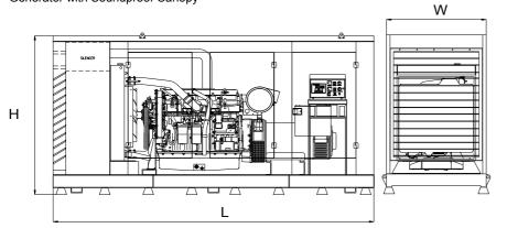
Length, L 4,1 m Heigth, H 2,45 m Width, W 1,4 m Weight, Total 4850 kg
