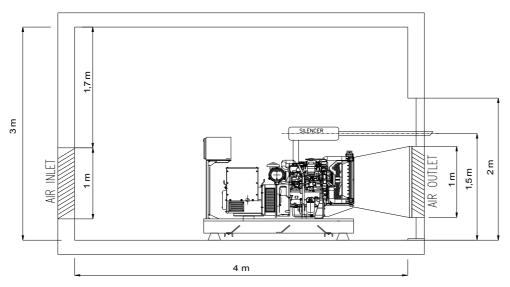
Above drawings dimensions and weights are only for guidence. For installation design of your specific application, necessary certified drawings, at site consultancy service as well as maintenance and installations manuals will be provided by Cukurova without any charge. Specifications may change without notice
