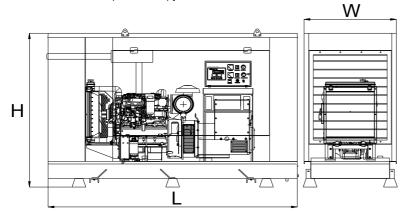
Length, L 2,6 m Heigth, H 1,85 m Width, W 1 m Weight, Total 1600 kg
